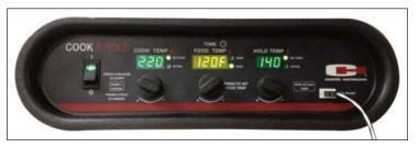
**EASY-TO-USE DIGITAL CONTROLS...** Control cooking and holding with separate dial controls and digital display. Cook according to time or according to product temperature with meat probe. Temperature range of 100°F to 200°F for hold cycle and 100°F to 325°F for cook cycle. Eighteen hour timer counts down in cook cycle. When cook cycle is over, cabinet automatically switches to hold cycle and timer counts up.
